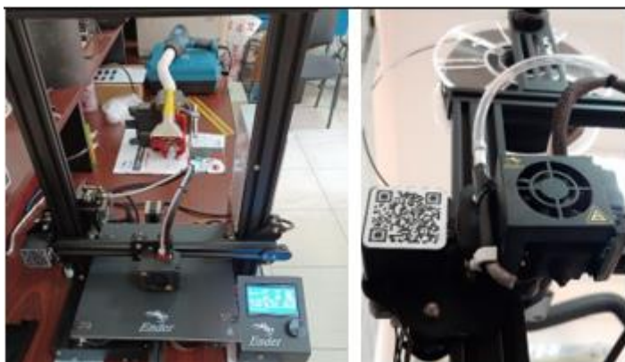
Figure 4. Creality Ender 3 printer modified for hybrid heating with additional hot-air jet
